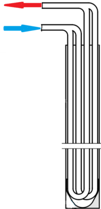
Fig.16. Ground vertical collector
